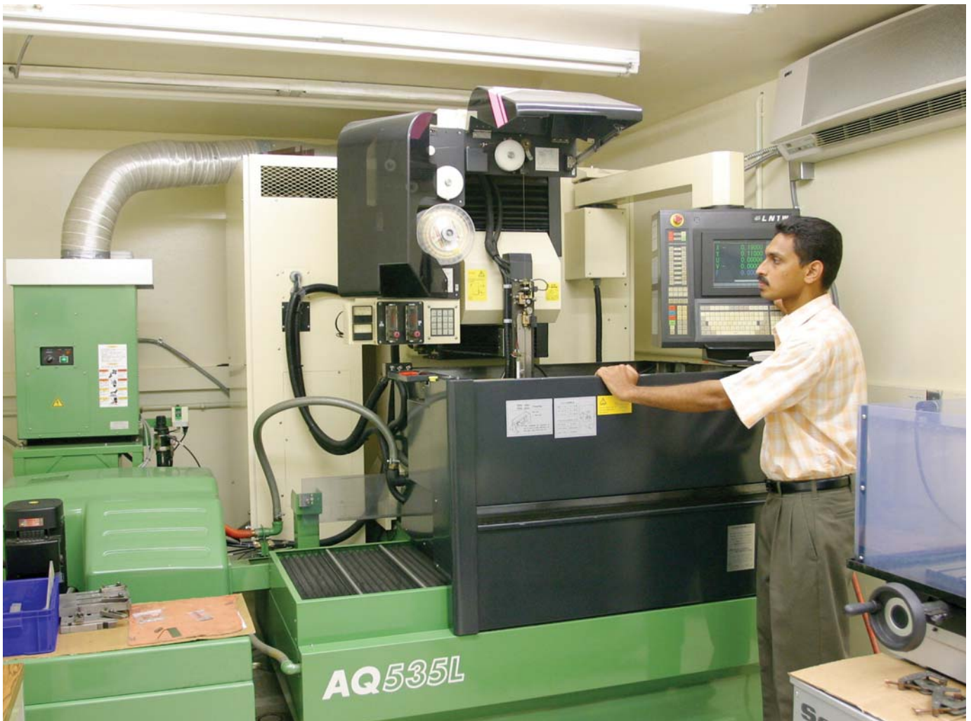
Biju Pulickal, EDM programmer, checks out A-1 Jay's Sodick AQ535L wire EDM to make sure it's running smoothly. The company operates 4 Sodick wire EDM machines and 1 Sodick K1C hole popper.
